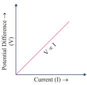
**Resistance** (R): It is the property of a conductor to resist the flow of charges through it.
