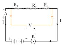
When two or more resistors are connected end to end, the arrangement is called series combination.
