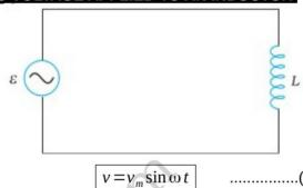
Apply KVL to the loop  $v = L \frac{di}{dt}$
