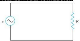
An AC source produce a sinusoidally varying pd across terminals.
