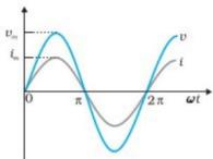
In a pure resistor, the voltage and current are in phase. The minima, zero and maxima occur at the same respective times.
