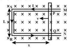
The magnetic flux  $\Phi_{\rm B}$  through the loop PQRS is,  $\Phi_{\rm B} = B \, L \, x$
