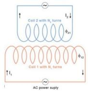
The **flux linkage** through the second coil is proportional to the current in the first coil
