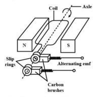
The basic elements of an ac generator are
