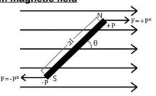
Two equal and opposite forces acting at the two ends of the dipole constitutes a torque.
