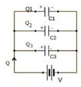
In a parallel circuit, the voltage is the same but the charges stored in the capacitors are different.
