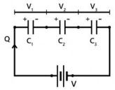
In a series circuit the charge (Q) stored in each of the capacitors is the same but the voltages across them are different.
