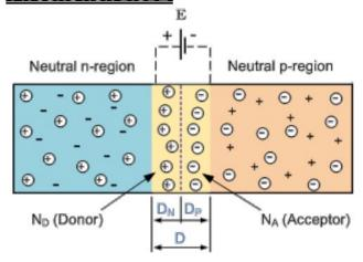
A p-n junction can be formed by adding a small quantity of pentavalent impurity to a p-type semiconductor or by adding a small quantity of trivalent impurity to an n-type semiconductor.
