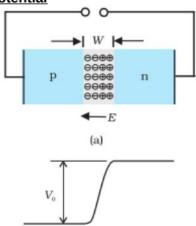
The loss of electrons from the n-region and the gain of electron by the p- region causes a difference of potential across the junction of the two regions. Since this potential tends to prevent the movement of electron from the n region into the p region, it is often called a barrier potential. The barrier potential of a Ge diode is 0.2Vand that of a Si diode is 0.7V.
