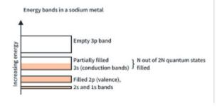
The highest occupied energy band (valance band) is not completely filled and acts as the conduction band. So the electrons are free to move within the band.
