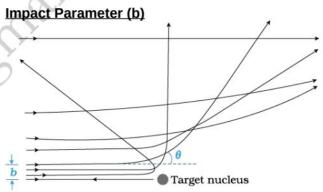
The impact parameter is the perpendicular distance of the initial velocity vector of the alpha particle from the centre of the nucleus.
