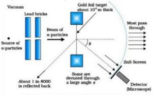
Schematic arrangement of the Geiger-Marsden experiment.
