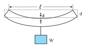
A beam of length l, breadth b, and depth d when loaded at the centre by a load W sags by an amount given by
