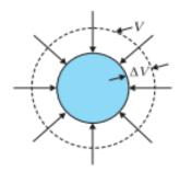
When a solid sphere placed in the fluid, the force applied by the fluid acts in perpendicular direction at each point of the surface.
