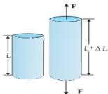
Longitudinal stress is defined as the restoring force per unit area when force is applied normal to the cross-sectional area of a cylinder.
