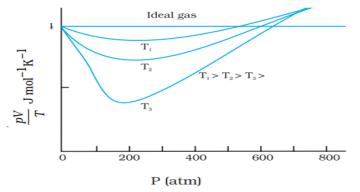
From graph it is clear that real gases approach ideal gas behaviour at low pressures and high temperatures.
