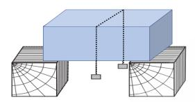
When the wire passes through the ice slab, ice melts at lower temperature due to increase in pressure. When the wire has passed, water above the wire freezes again. This phenomenon of refreezing is called **regelation**.
