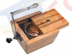
It consists a metallic vessel and stirrer of the same material like copper or alumiunium. The vessel is kept inside a wooden jacket which contains heat insulating materials like glass wool etc. The outer jacket acts as a heat shield and reduces the heat loss from the inner vessel. There is an opening in the outer jacket through which a mercury
