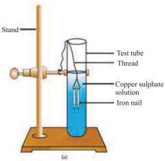
The iron nail becomes brownish in colour by deposition of Cu and blue colour of CuSO<sub>4</sub> changes to dirty green colour due to formation of FeSO<sub>4</sub>.
